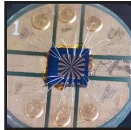
**Graphene device on chip carrier**
