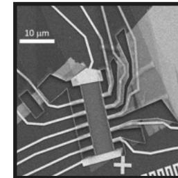
**2D spin Hall effect and thermoelectric device**
